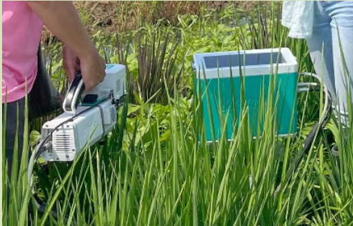
Collecting gas exchange measurements from rice plants in the field.
